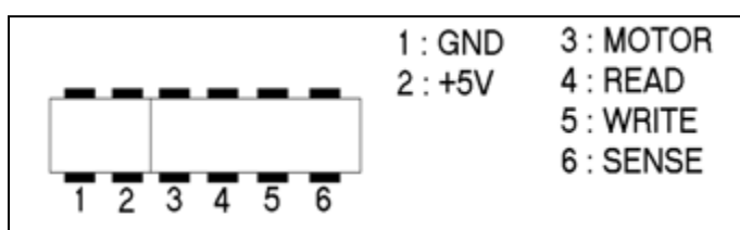
Figure 1. C2N 1530 connector pinout
