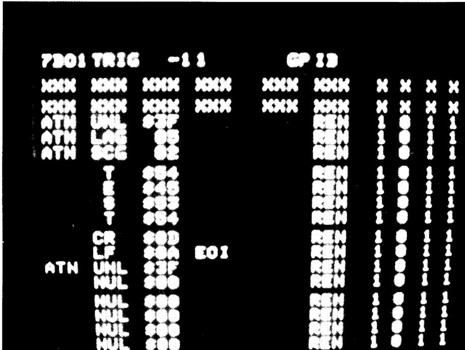
Figure 7-23. The image of the DF2 Display Formatter when the logic analyzer is triggered on the LAG (Listen Address Group). See text for the OPEN and PRINT statements that provide data for the display.
